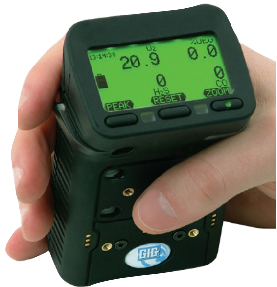
Figure 1: Always allow all of the sensors installed in your instrument to stabilize completely in fresh air BEFORE making a fresh air zero adjustment
