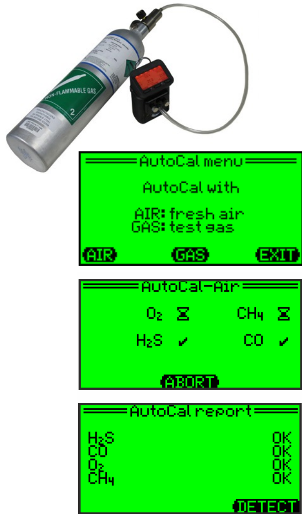
Figure 4: GfG instruments can be automatically fresh air zeroed or calibrated by means of a simple "AutoCal" procedure, (press "Air" to make an automatic fresh air zero adjustment, "Gas" to make a span calibration adjustment, or "Exit" to return to normal operation).
